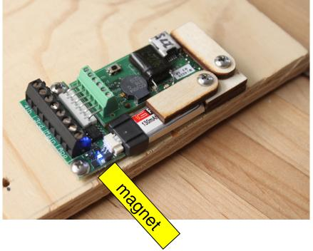
The switch changes state when either end of the magnet leaves the vicinity of the sensor. To turn the Raven on or off, put either end of the magnet close to the sensor and then remove it.
