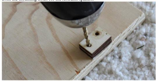
If a 3/32" drill bit is used, the included 4-40 screws will thread themselves securely into the plywood. If the screws are to be retained with the included nuts on the back side of the sled, use a 7/64" or 1/8" bit to provide clearance for the threads. The restraint spacers can be glued to each other and glued to the sled if desired. Install the battery restraint with 1 screw to fix it into position for locating the other holes.
