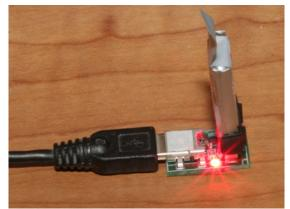
To use the Featherweight USB Battery Charger, plug the battery in to the board, the connect the USB cable to the board, and finally to either a USB port on your computer, or a USB wall wart. The LED on the board will be red while the battery is charging, and will turn orange when charging is complete.
