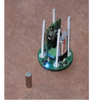
voltage can prevent the Raven from powering up properly when an external power source is re-applied. After turning using the magnet to turn the Raven off, use the magnet or another conductive item to discharge the capacitor, as shown at left. For a Raven 2, this step is not necessary.
