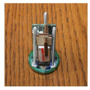
the capacitor notch to the rear, the wider portion of the second piece is to the left, as shown in the picture above. If this piece is reversed, the restraint will not fit properly around the USB port on the Raven.
