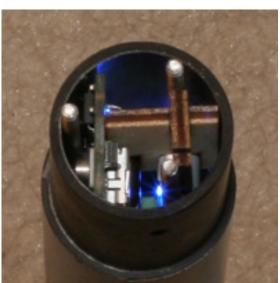
Drop the bulkhead with the rods through the tube with the coupler, so that the rods poke through the coupler. If the battery restraint has not been glued onto the passive bulkhead, install it now. Install the passive bulkhead over the threaded rods.
