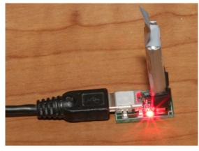
finally to either a USB port on your computer, or a USB wall wart. The LED on the board will be red while the battery is charging, and will turn orange when charging is complete.
