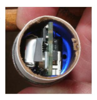
Important: Align the two bulkheads so that they are facing the same direction. If the labels are not facing the same direction, the charges will be connected to the wrong terminals. Attach the shock cord and deployment charges as you did for the other end of the av-bay. Completed av-bay shown below.
